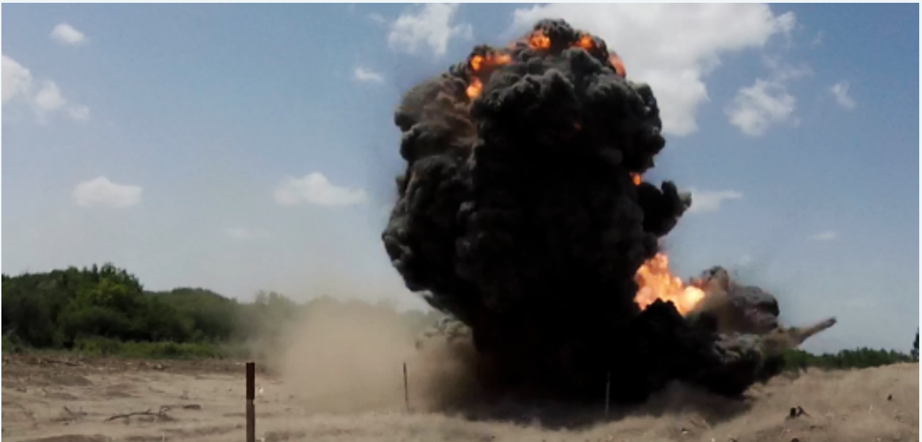
EXPLOSION OF TM-62 ANTI-TANK MINE (8 KG TNT)
