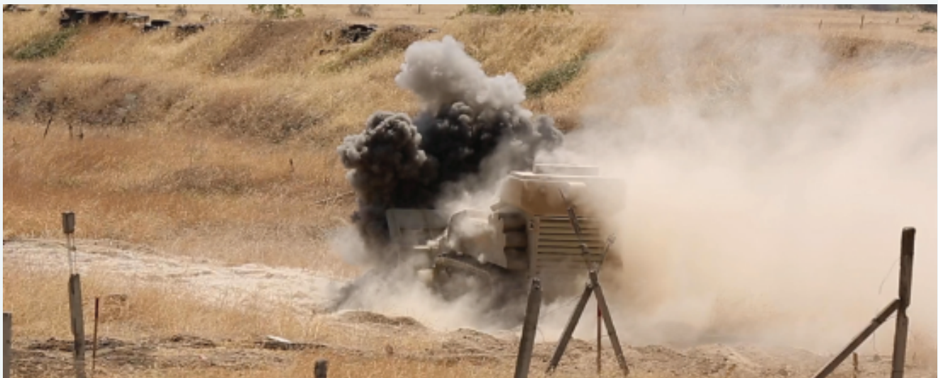
EXPLOSION OF TM-57 ANTI-TANK MINE (6,5 KG TNT)
