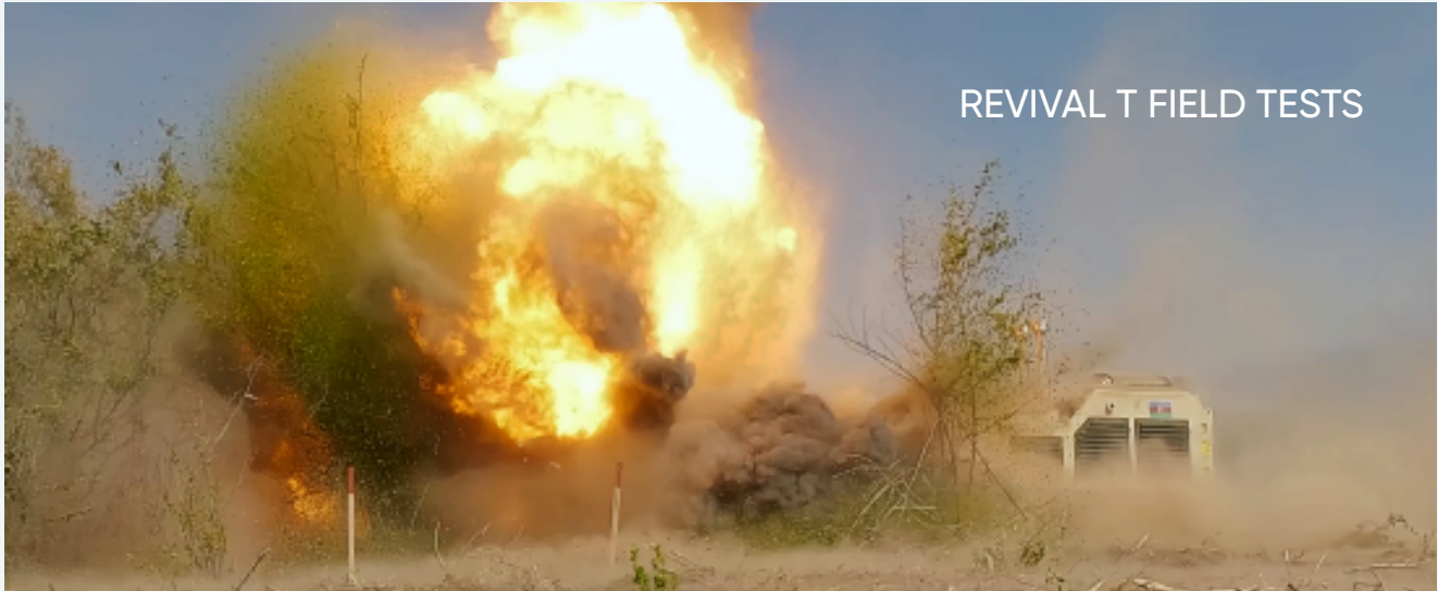
EXPLOSION OF TM-62 ANTI-TANK MINE (8 KG TNT)
